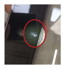
Underpainting of the screen printing causing clearances is unacceptable.
