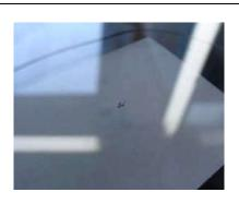
Defect acceptable if it occurs in the edge zone of the glass and if it is a maximum of 1 defect not exceeding Ø<0,8mm.
