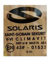
The windshields should bear the appropriate approval mark and the Solaris logo. Approval mark legible from the outside of the vehicle, intermittent writing not permitted. The design of the approval mark must be approved between the supplier and Solaris Bus & Coach sp. z o.o.
