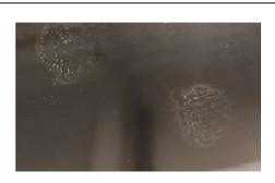
Unacceptable defect - these are all kinds of dirt from the production process, fingerprints, cork marks on the surface. The glass surface should be clean, free from any contamination or residue from the production process.
