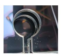
Defect acceptable in the edge zone, a maximum of 2 pieces with a diameter of 1.5 mm, a minimum of 200 mm apart.
