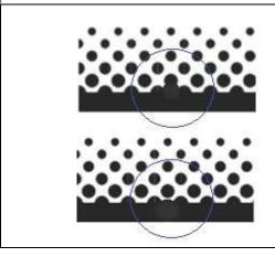
Connected dots (converging dots in screen printing) allowed between two dots of the first row of half dots or between two dots of a row of half dots and a dot of the first row of full dots are allowed under the condition: max. 2 defects / min. 500 mm (measured on the outline of the glass sheet).
