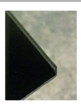
A defect is permissible if the cut does not exceed 2 mm.
