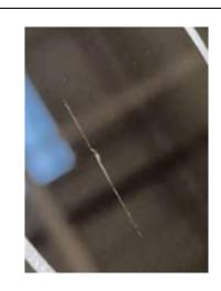
Deep scratches - all kinds of scratches and abrasions that can be felt with the fingernail.
