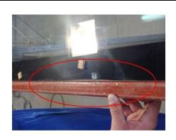
A defect is permissible if the deviation of straightness is a maximum of +/- 1 mm and if the difference in the lengths of the diagonals is a maximum of 2 mm.
