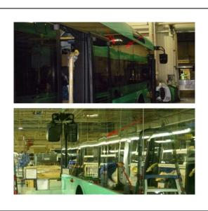
Glazing with a wavy surface is unacceptable.
